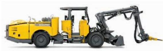
Scaling involves the removal of excess loose rock on roofs and walls after blasting – an essential task for safety.
