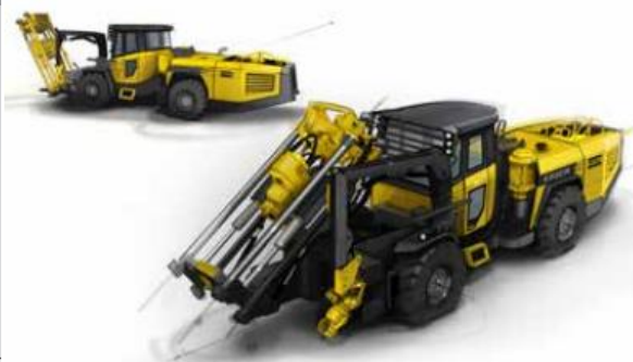
Figure 8: The Easer machine is a flexible rig for small diameter raises.
