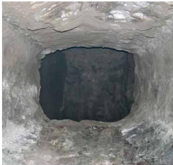
Fig 5: Opening raise, offering swell volume for production blasts.
