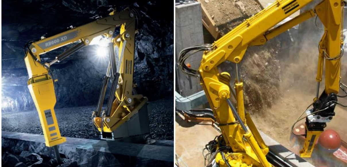
Pedestal Boom Systems in action, over a grizzly and over a crushing station (right), which demands a longer reach.
