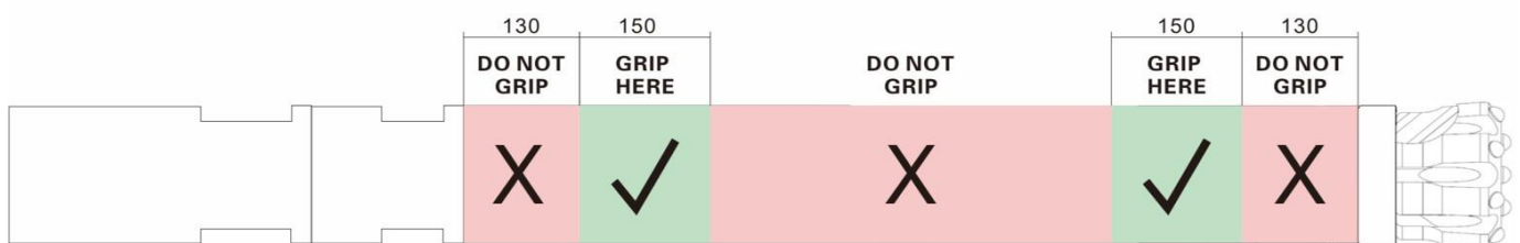
Figure 1: Gripping Locations for BD DRILL Reverse Circulation Hammer Lubrication
